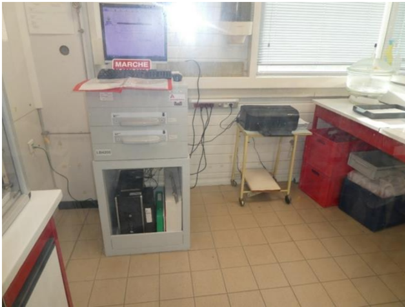
Figure 30. Alpha/beta counter for water samples at the Orano site laboratory
