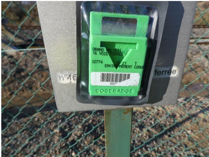
Figure 9. TLD dosimeter on the site fence
