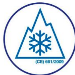
Figure 18: Alpine symbol (3-PMSF) used for marking severe use snow tyres according to UNECE Regulation No 117.
