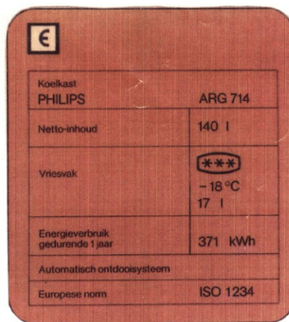
Figure A-3 The 5 energy labels tested by the University of Leiden - The old EC label format in compliance with Directive EEC 79/530
