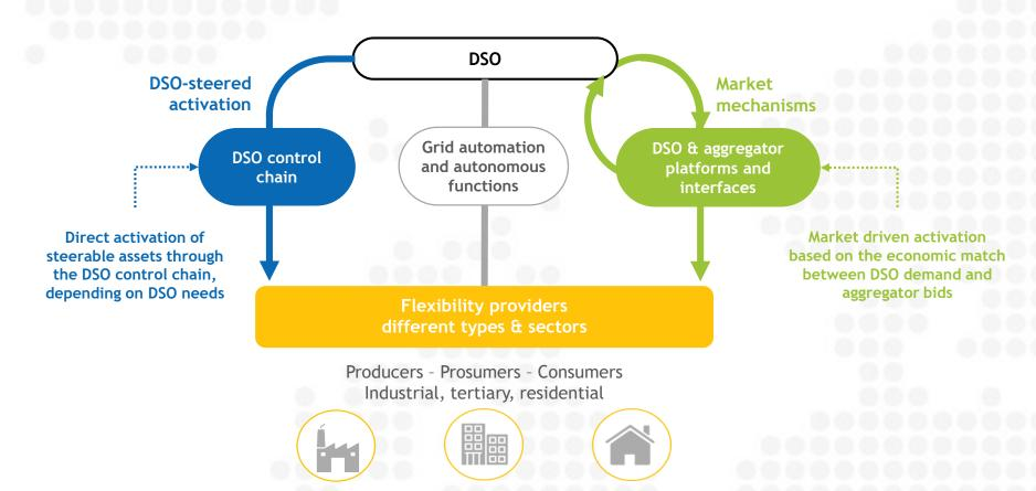
Batteries, EV, thermal inertia, residential heating, sector coupling, DER curtailment, ...
