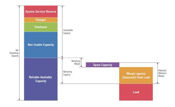
Figure 1 ENTSO-E schema for analysing generation adequacy
