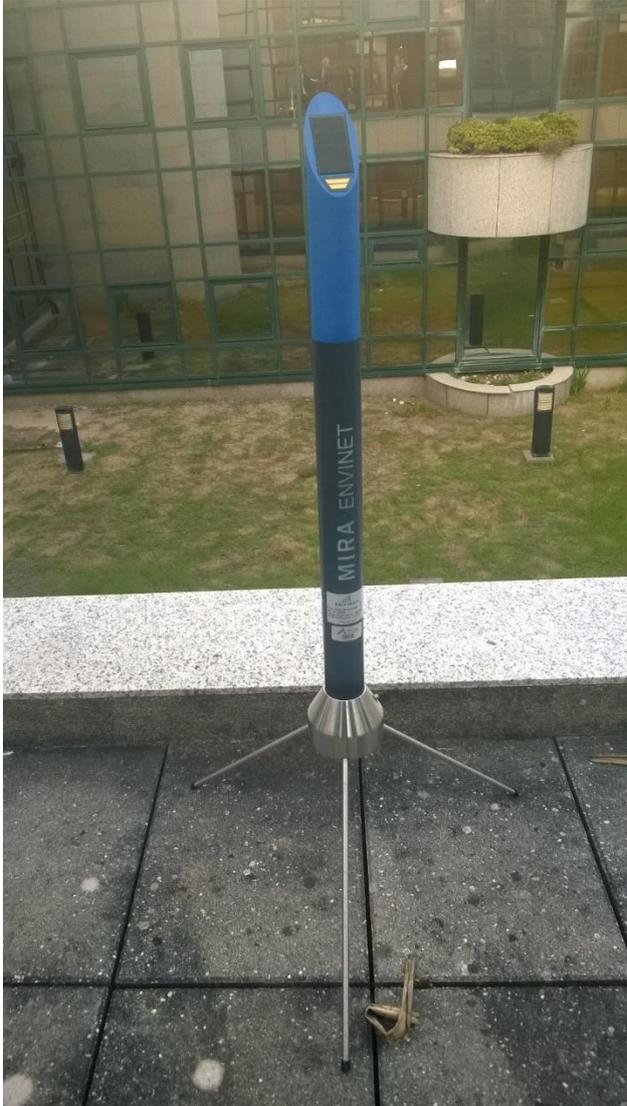
**Figure 8. Envinet MIRA mobile radiation dose rate monitor**
