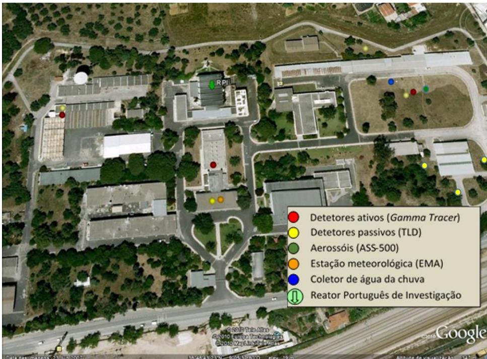
**Figure 2. Map of IST campus with the identification of the monitored sites: active detectors (red circles), TLD (yellow circles), high volume aerosol collector (green circle), meteorological station (orange circle), rain water collector (blue circle) and the Portuguese Research Reactor (green arrow)**
