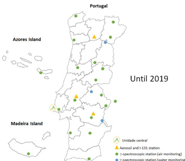
**Figure 5. RADNET stations deployment by the end of 2019**
