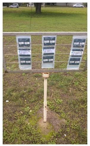
*Figure 11. TLD dosimeters of the IST environmental radiation surveillance programme*
