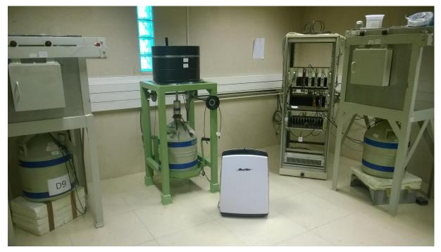
Figure 9. IST laboratory gamma spectroscopy systems
