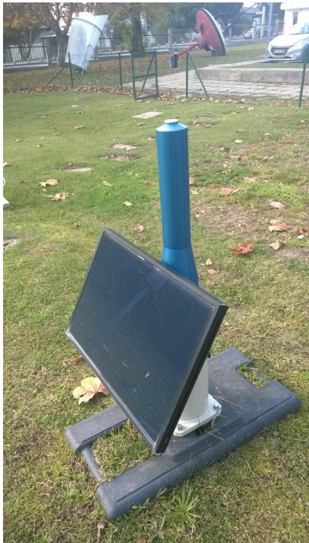
**Figure 7. Envinet SARA dose rate monitoring station with a solar panel**
