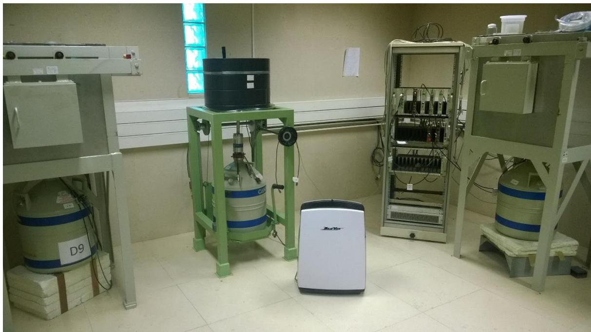
**Figure 9. IST laboratory gamma spectroscopy systems**
