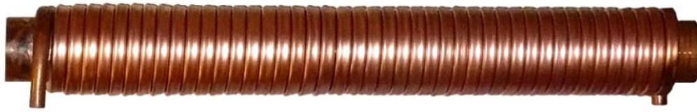
Figure 4.8. The so-called pipe-in-pipe heat exchanger type for utilising the heat of the waste water. Sewage flows around the cold domestic water pipe
