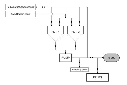
1.2 <u>CMT - collection monitoring tanks - discharge system (Magnox dissolution plant)</u>
