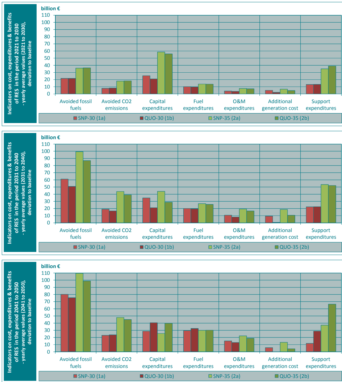
Figure IV-24: Indicators on yearly average cost, expenditures and benefits of RES at EU 28 level for all assessed cases, monetary expressed in absolute terms (billion €) per decade (2021 to 2030, 2031 to 2040, and 2041 to 2050)
