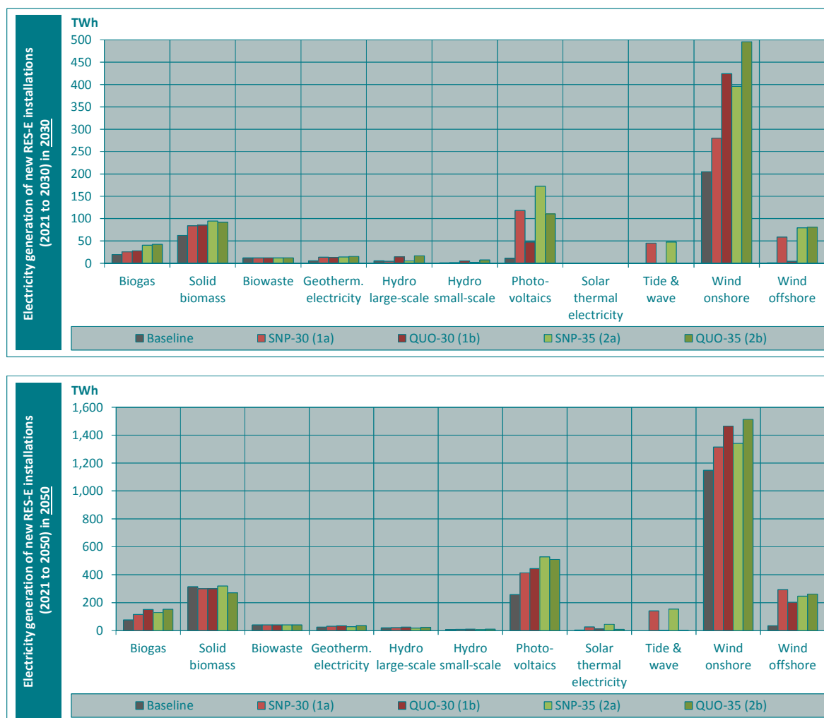
Figure IV-23: Technology-specific breakdown of RES-E generation from new installations by 2030 (top, incl. new installations from 2021 to 2030) and by 2050 (bottom, incl. new installations from 2021 to 2050) at EU 28 level for all assessed cases
