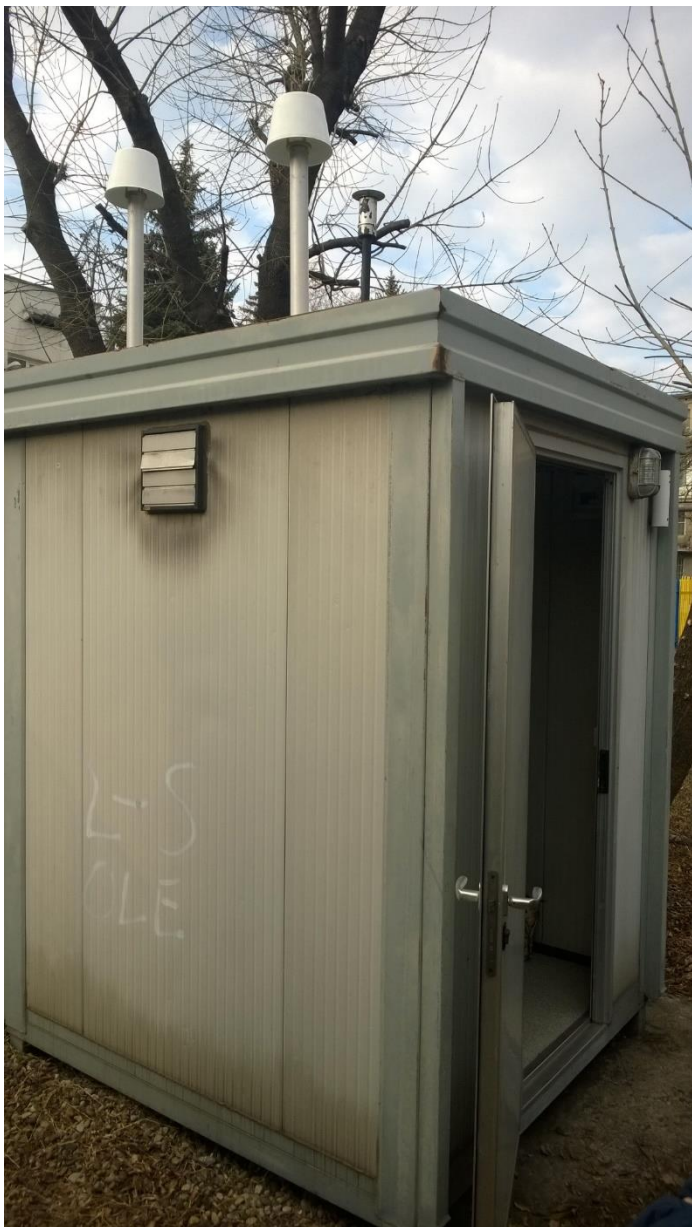
Figure 3. High volume air sampling container in Nadezhda, Sofia, for atmospheric radioactivity monitoring
