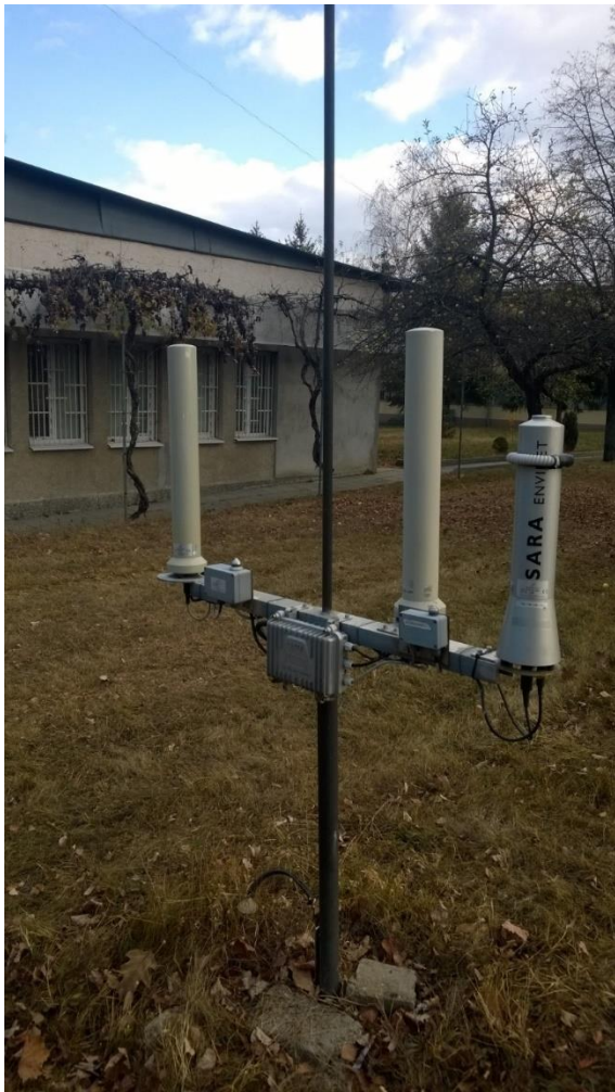
Figure 2. Envinet SARA automatic radiation monitoring station with a control source ring
