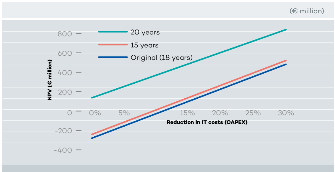
Germany CBA: Impact on project NPV of cost reductions in IT capital costs
