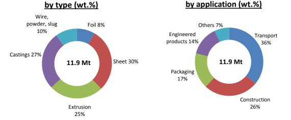
*Figure 18. EU consumption of aluminium (source: European Aluminium Association, 2015)*
