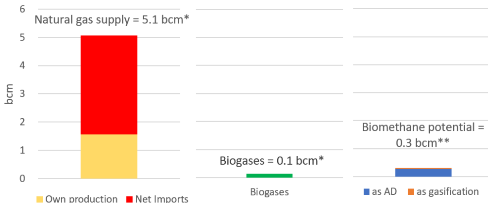
Figure 1 Comparison of current natural gas supply, biomethane production and potential in Slovakia (2021) (sources: Eurostat: Energy Balances, 2022*; Guidehouse: Gas for Climate Report 2022**)
