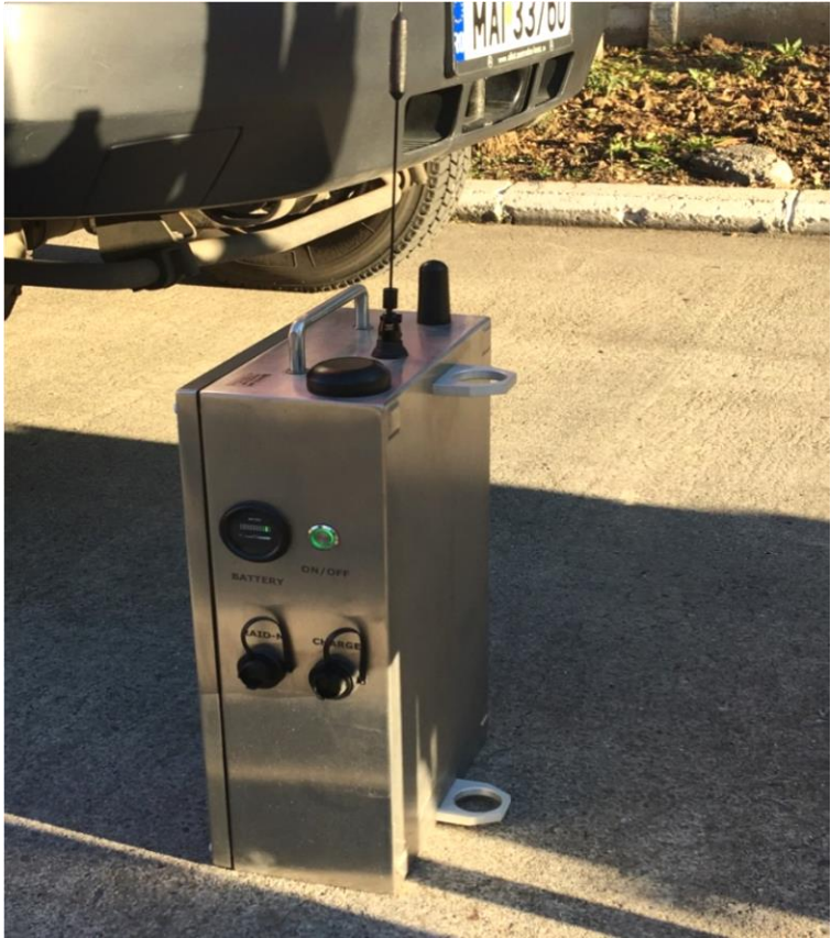
Figure 6. Independent mobile radiation dose rate monitor EXATEL ARGU-SAT
