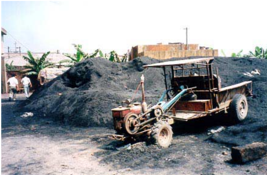
Figure 12 Char waste from rice husk gasification creating a waste disposal problem
