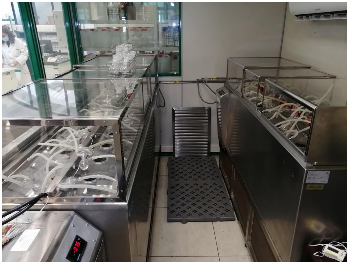
Figure 5. Electrolytic low-temperature enrichment system for H-3 analysis
