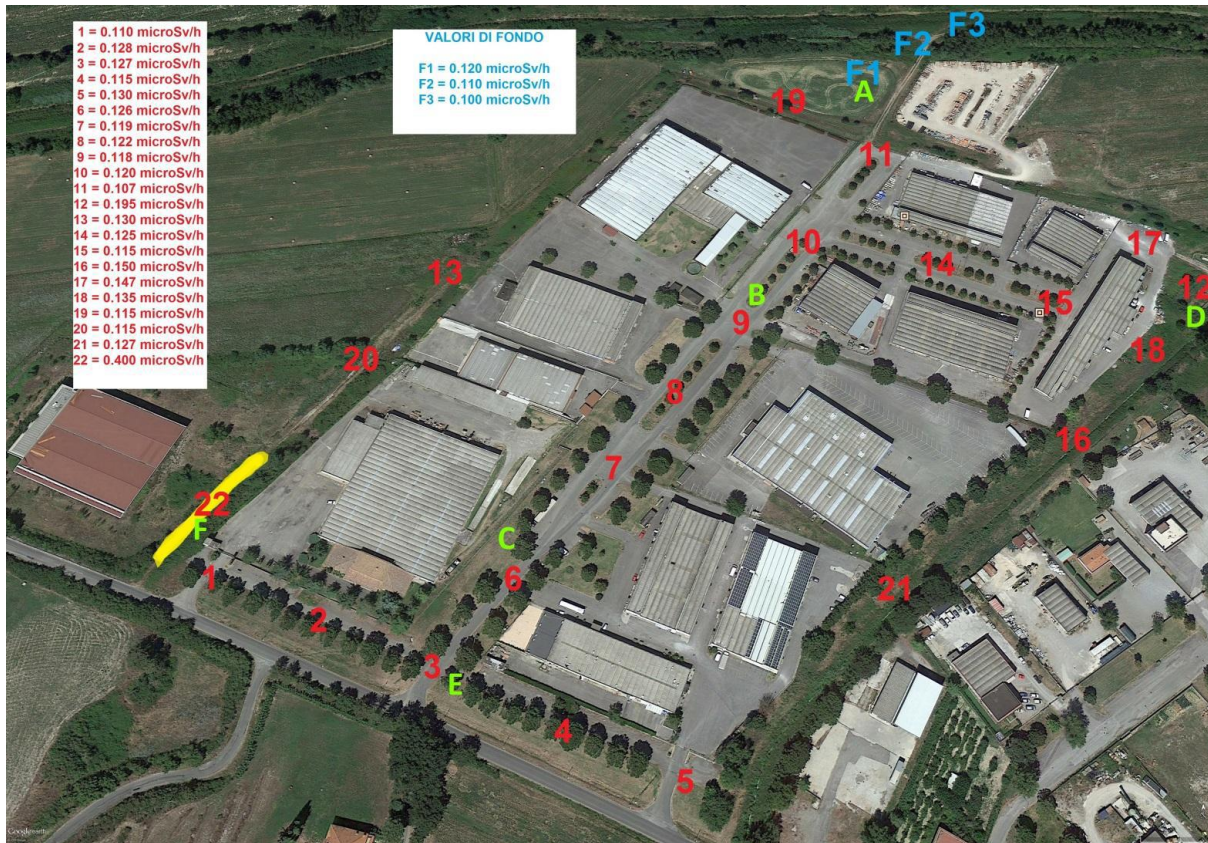
Figure 3. Colonna di Fabro site dose rate monitoring points
