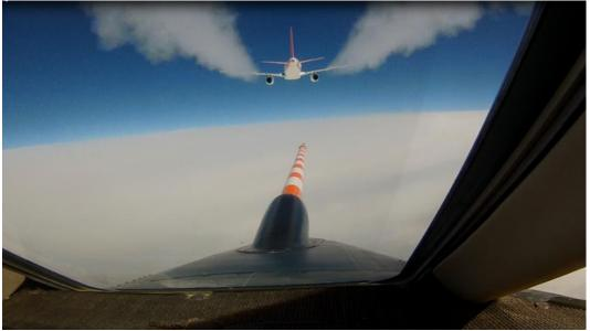
DLR's research aircraft Falcon measuring emissions and contrails from biofuels in the wake of DLR's ATRA (Advanced Technology Research Aircraft) during a measurement campaign in fall 2015.
