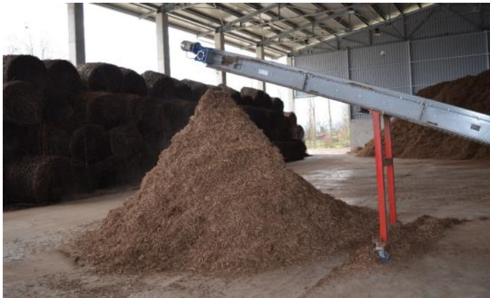
Figure 41: residual vine residue is chipped and transferred to a heat conversion plant onsite
