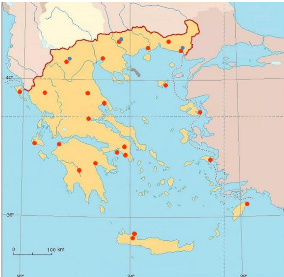
Figure 2: Locations of measuring stations: ambient gamma dose rate meters (dark/red spots); air monitors (blue spots).
