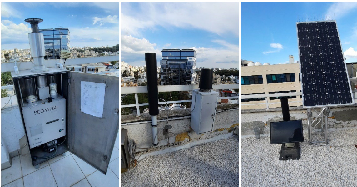
Figure 2. Continuous monitoring equipment at the DLI office roof (Sven Leckel SEQ47/50 low-volume air sampler, BITT RS04/X Gammameter with data logging unit and ENVINET SARA Dose rate monitor)
