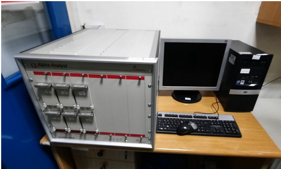
Figure 10. Alpha spectroscopy system at the SGL radiological laboratory
