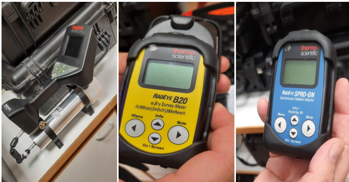
Figure 6. Hand-held radiation monitors at the DLI (RIIDEye NaI Nuclide identification device, RadEye B20 Survey meter and RadEye SPRD-GN Spectroscopic radiation detector)
