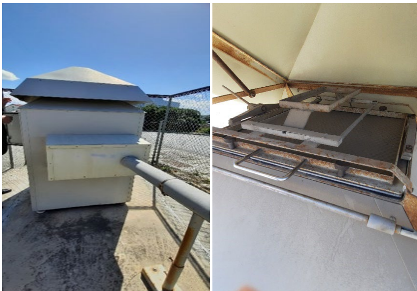
Figure 4. High-volume air sampler POLON-IZOT ASS-500
