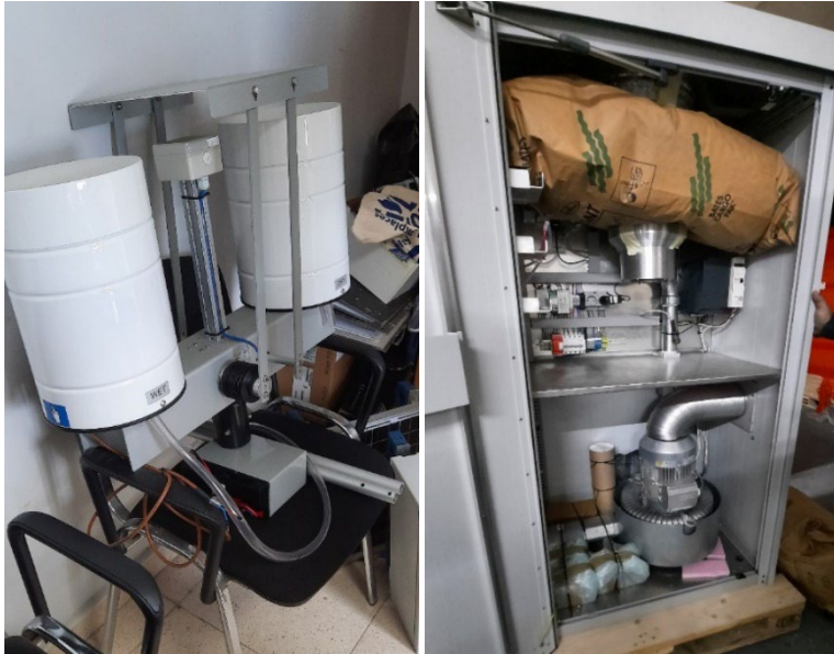
Figure 8. New monitoring equipment, which are being implemented for operational use (Wet/dry atmospheric deposition sampler and medium-volume continuous air sampler)
