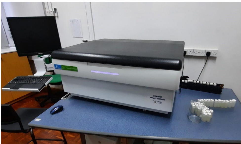
Figure 11. Liquid scintillation counter at the SGL radiological laboratory
