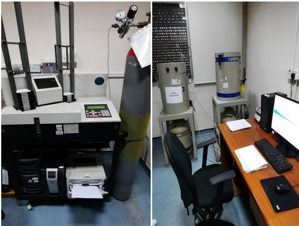
Figure 9. Automatic proportional counter system for measuring air filters and two HPGe-gamma spectrometers at the SGL radiological laboratory
