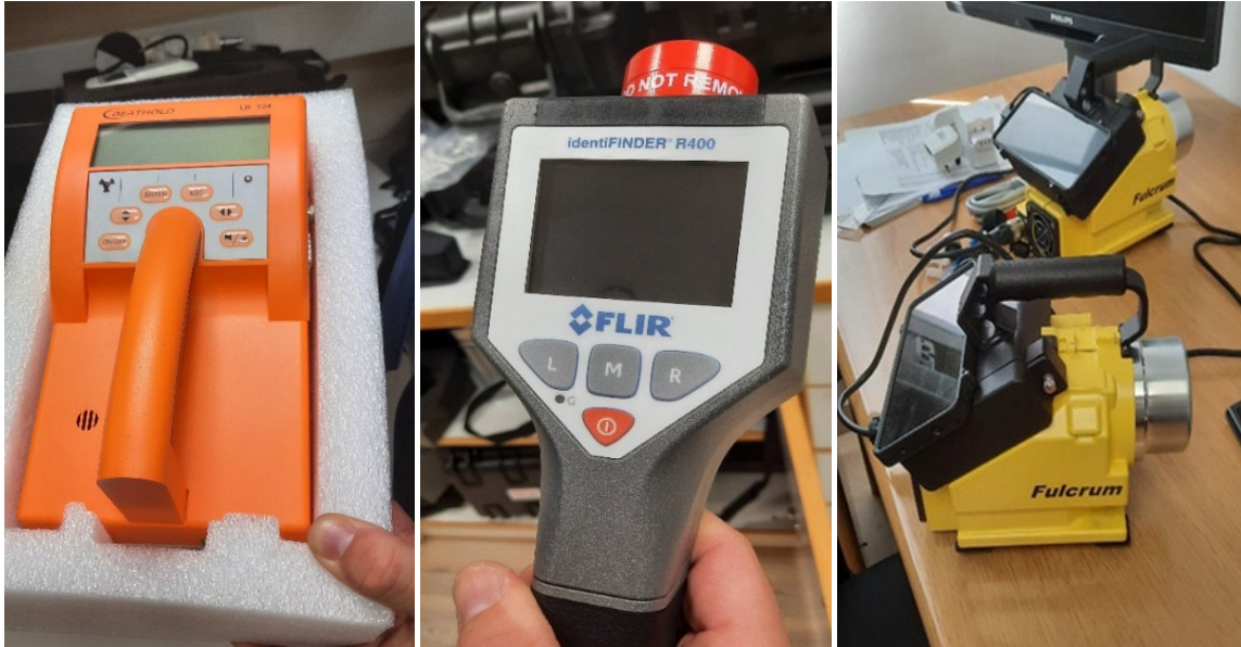
Figure 7. Hand-held radiation monitors at the DLI (Berthold LB 124 Surface contamination monitor, Flir IdentIFINDER R400 Nuclide identification device and Fulcrum electrically cooled portable HPGe-gamma spectroscopy systems)
