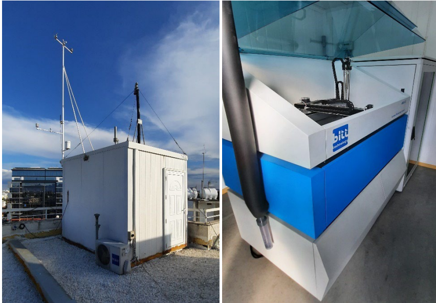
Figure 3. Continuous monitoring equipment at the DLI office roof (BITT AMS02 automatic radioactivity monitoring station)
