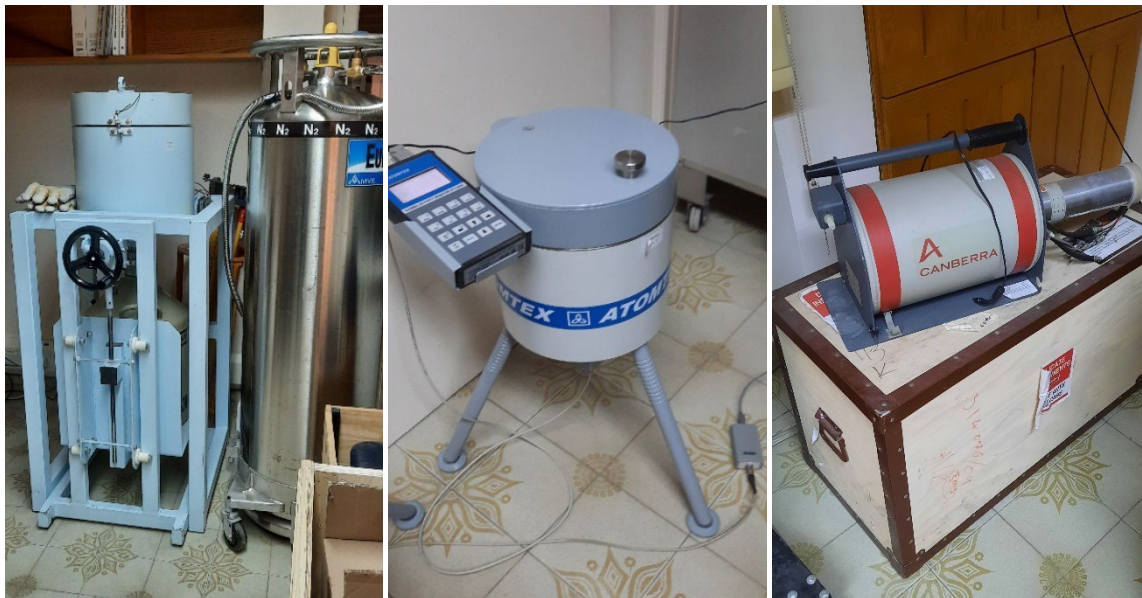
Figure 5. Counting equipment at the DLI office (Ortec HPGe-detector, Atomtex NaI-detector and Canberra portable HPGe-detector)
