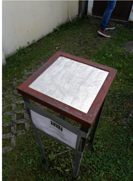
Figure 18. IMROH dry deposition collector
