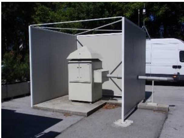
Figure 5. High-volume air sampler at IMROH in Zagreb
