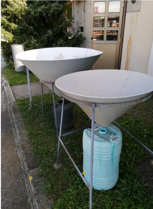
Figure 17. IMROH wet deposition collectors
