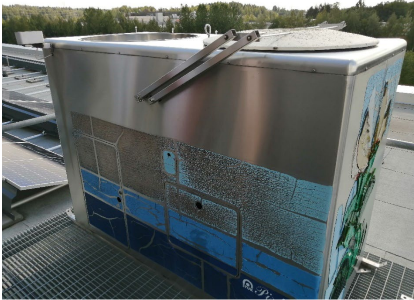
Figure 20. Automatic dry/wet atmospheric deposition collector 'Pirkko' at STUK
