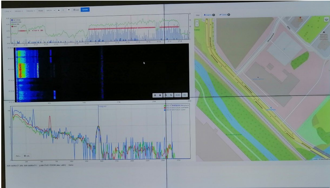
Figure 14. USVA-network waterfall display of radiation spectra with GPS positioning
