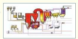
The plant operates a waste pre-treatment facility, which involves crushing of waste and separation of metals and inerts, drying and bio-stabilisation of sludge and grinding of coal before the materials enter the combustion chamber. Combustion takes places in a circulating fluidised bed with the addition of limestone. The energy in the fuel is used to produce superheated steam, which drives the steam turbine of the plant. Electricity is fed to the national grid.
