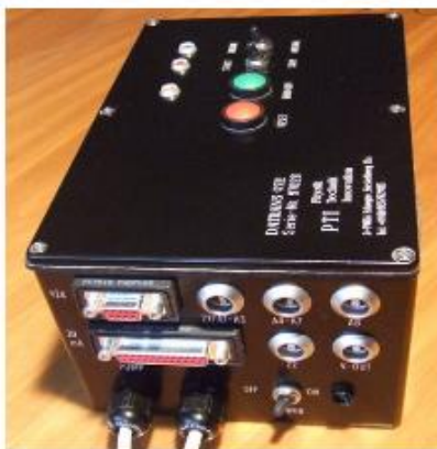
Datalogger/Interface DATRANS 97E Degree of Protection IP 65
