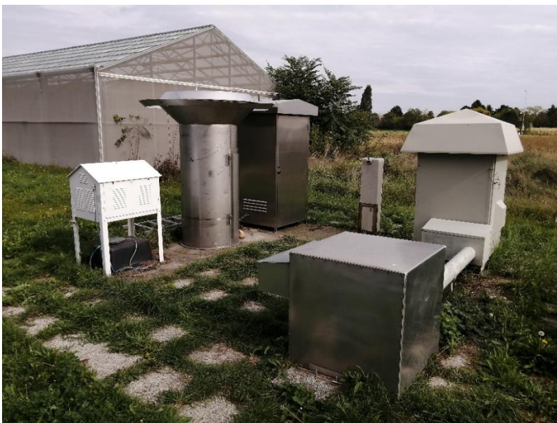
Figure 15. Atmospheric sampling equipment at the AGES laboratory site (from left: small-volume iodine sampler, large deposition sampler, medium-volume air sampler and a high-volume air sampler)
