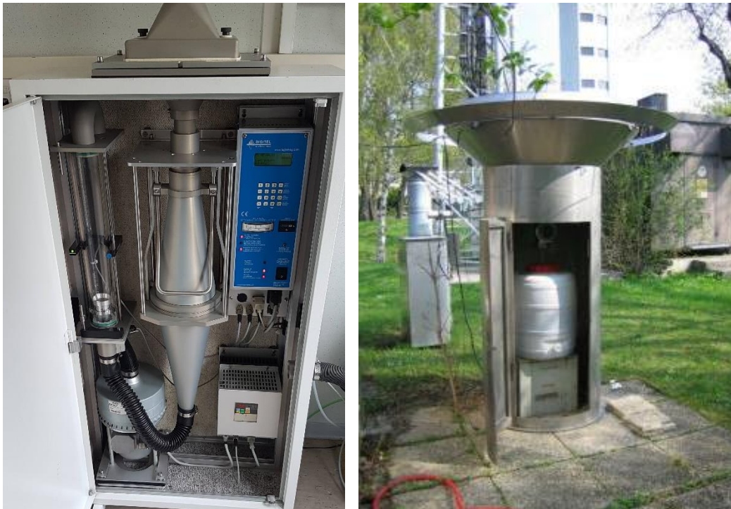
Figure 9. Left: Cascade impactor - Digital/ Tisch Environmental Inc.; Right: Large dry/wet deposition collector
