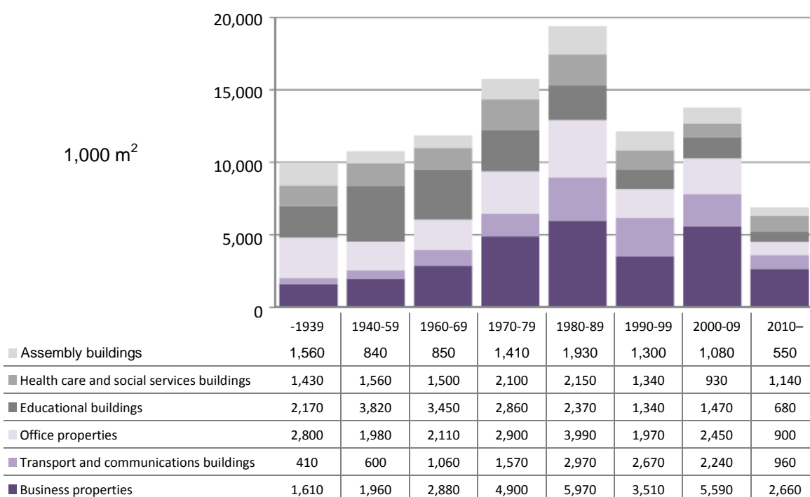
Figure 4. The gross floor area and age structure of commercial and public buildings in Finland. The gross floor area of commercial buildings is 60 million square metres and that of public buildings is 40 million square metres. Source: Statistics Finland, Buildings and free-time residences, 2016.
