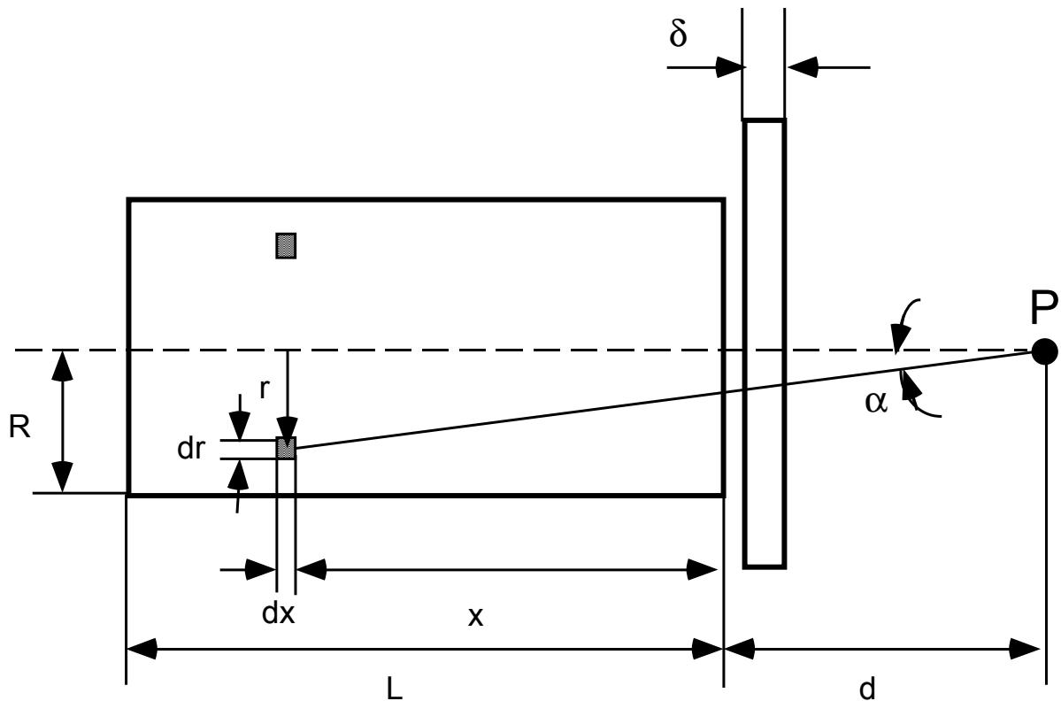
**FIGURE 1 Diagram showing parameters for calculating flux  $\phi$  from gamma sources**
