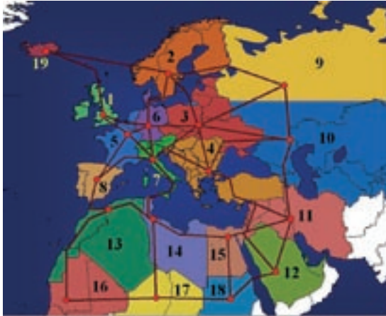
Figure 30: Schematic representation of potential electricity transmission paths for an intercontinental overlay transmission system
