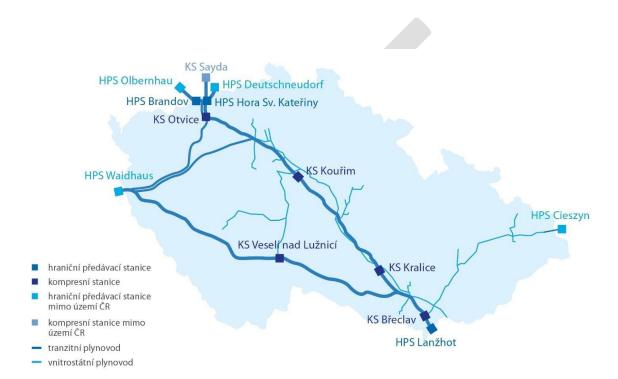
Fig. No. 1: The Gas System of the Czech Republic
