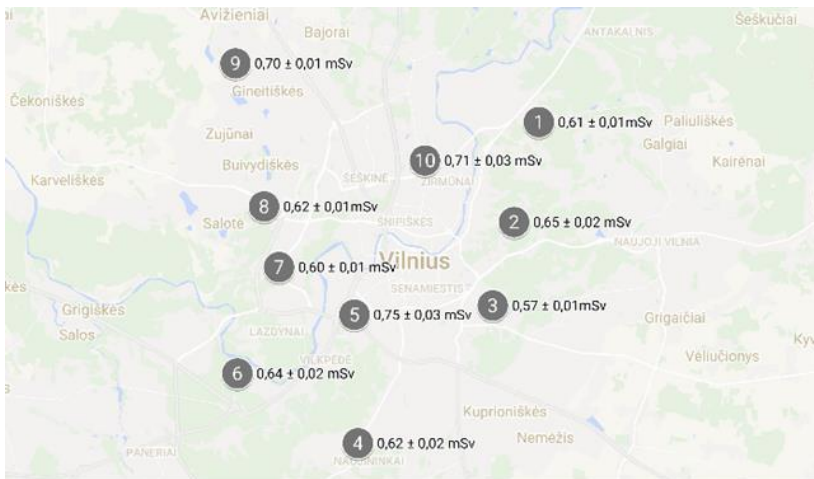
Figure 2. Monitoring points and average annual ambient dose equivalent in Vilnius in 2015
