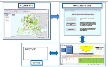
Schematic representation of Database Analysis/Interrogation Tool, showing the GIS (at the top) and the StoreFit Monte Carlo analysis tool (bottom). Arrows indicate data exchange between the separate elements of the tool.
