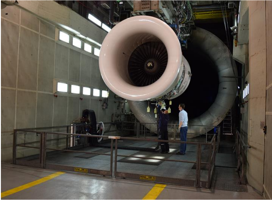
Figure 57: EVE engine in test rig chamber
